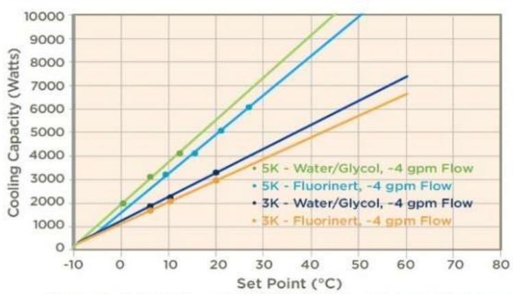
Note: Configurations using the large pump at high pressure and flow can reduce cooling capacity as much as 1200 Watts
