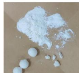
6) Human premolar after grinding at 7500 rpm, 1x 20s
