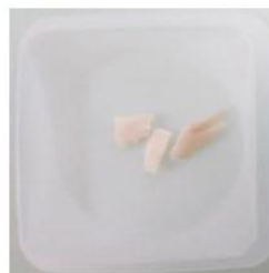
3) 200mg of marrowbone before grinding with Precellys Evolution
