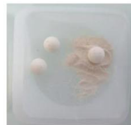
4) 200mg of marrowbone after grinding at 75000 rpm – 10x20s (1 min break)
