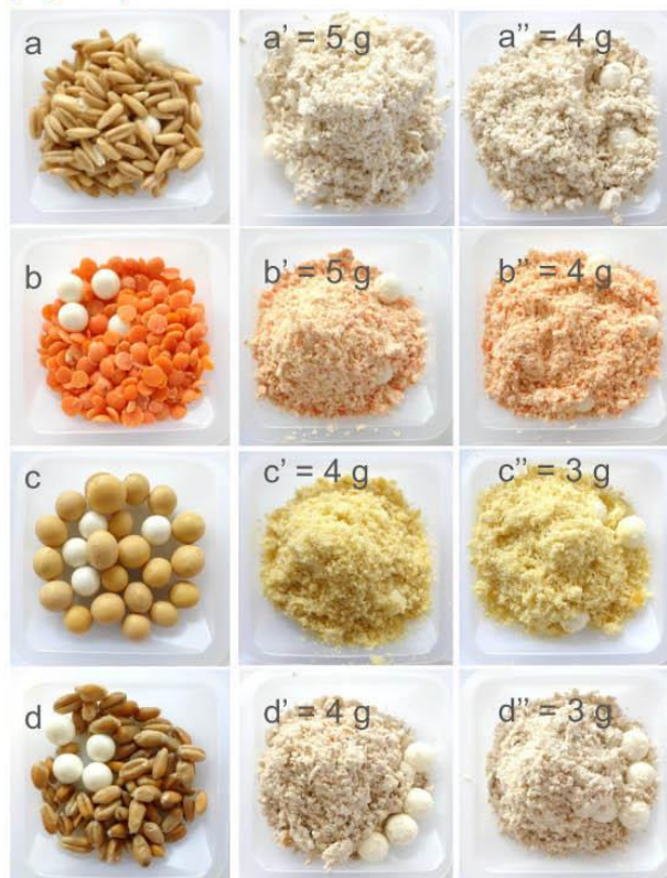
Figure 1: a) Oat seeds b) Coral lentils c) Soybean, d) Grain of wheat (3, 4 or 5g) before/after (" ; ") grinding using Precellys® Evolution.
