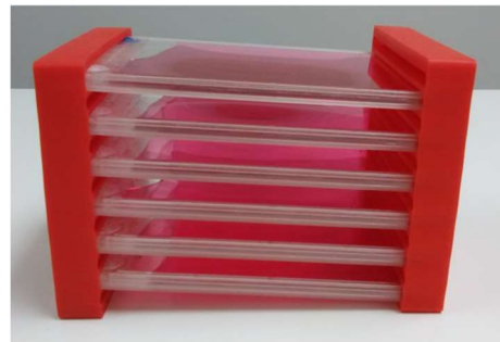
The preferred horizontal configuration with the top end slightly higher than the bottom end.
