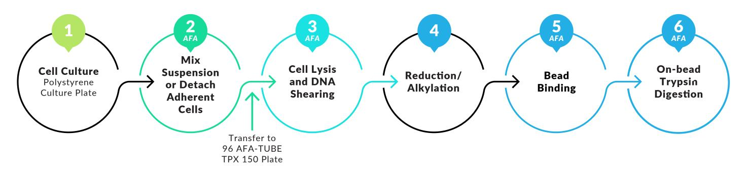
**Figure 2. AFA-enabled Workflow.** AFA conditions for cell detachment, cell lysis, DNA shearing, and protein extraction were developed with HCT 116 cells (*Figure 1*). AFA conditions for bead-binding and on-bead trypsin digest were developed using K562 protein extract (*Figure 3*).
