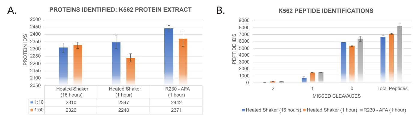
**Figure 3. LC-MS Analysis of Tryptic Digestion of K562 Cell Protein Extract.** K562 protein extract was bound to magnetic beads using AFA-enhanced mixing and then digested with trypsin (using trypsin to protein ratios of 1:10 or 1:50) by either incubating in a heated shaker (1 hour or ON at 37 °C) or by applying AFA in an R230. High confidence protein identifications are shown (**A**) as well as a comparison of missed cleavages and peptide identifications between digestion methods (**B**).
