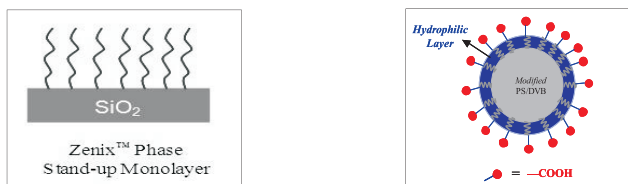
Figure 1. Phase structures for both the surface of Zenix™ SEC and Antibodix™ WCX.
