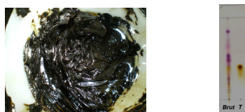
Figure 1 Crude extract of Artemisia annua L. And TLC of crude mixture and standard of artemisinin
