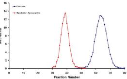
**Figure 1:** Variation of HPLC Peak Area of 1 min Fractions for a CPC separation of Lysozyme and Myoglobin using a 500ml rotor. Separation Conditions: Rotor speed 2000rpm, Mobile phase flow 10ml/min, fraction volume 10ml, sample loading 40ml (10%CV), sample concentration 2.2+2.2 mg/ml, phase system 12.5% w/w PEG-1000: 12.5% w/w K<sub>2</sub>HPO<sub>4</sub> ATPS system.
